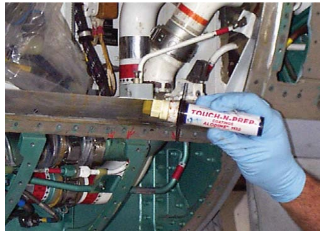
Figure 5-3. Application of TNP Pen on Aluminum Substrate
