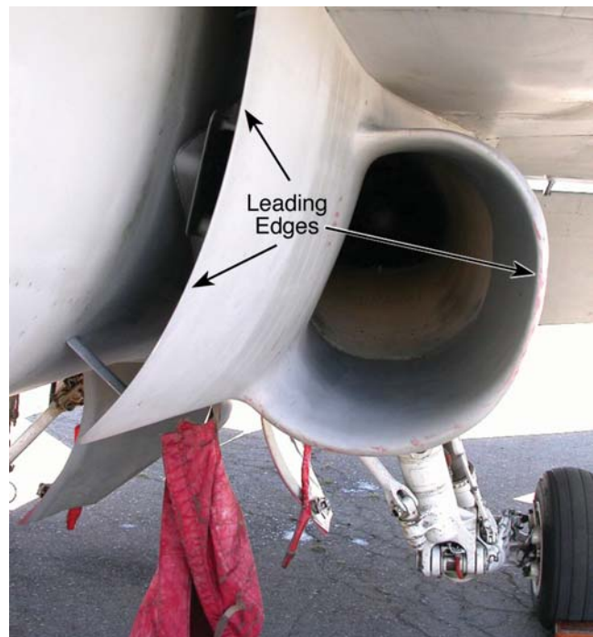
Figure 3-15. Corrosion Prone Points of Air and Engine Inlet
