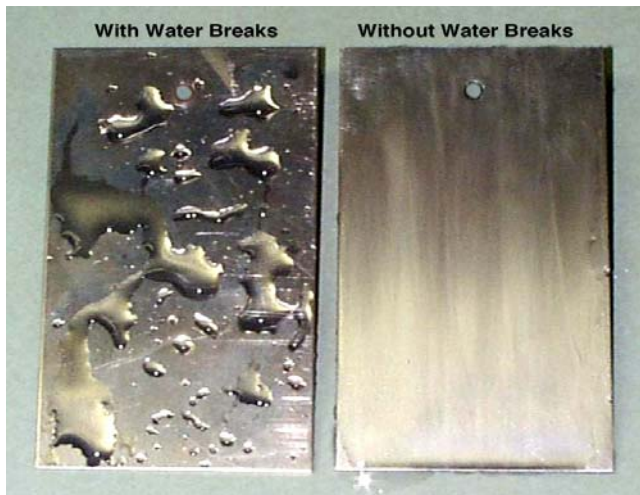
Figure 5-1. A Water Break-Free Surface Compared to One with Breaks
