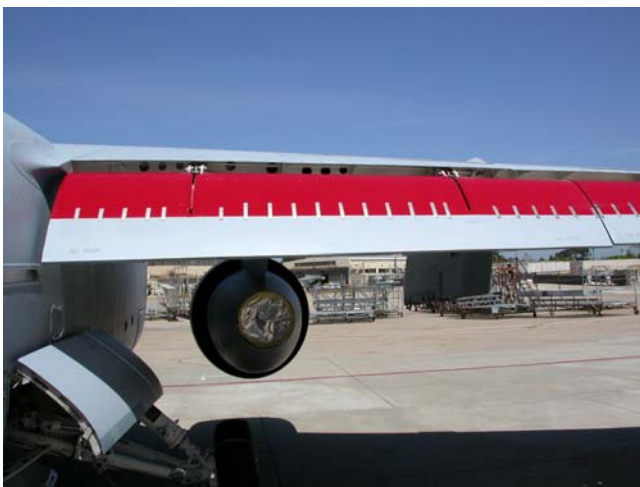
Figure 3-12. Flaps Lowered to Expose Recess Areas
